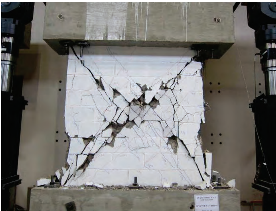
Figure 4-2 Failure of a shear-dominated wall (Wall UT-PBS-02 tested by Ahmadi, 2012).
