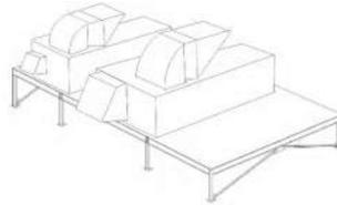
Equipment support platform supporting two mechanical components
